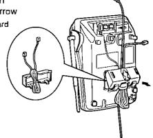
4 Connect the telephone line cord Mount the unit, then slide down
